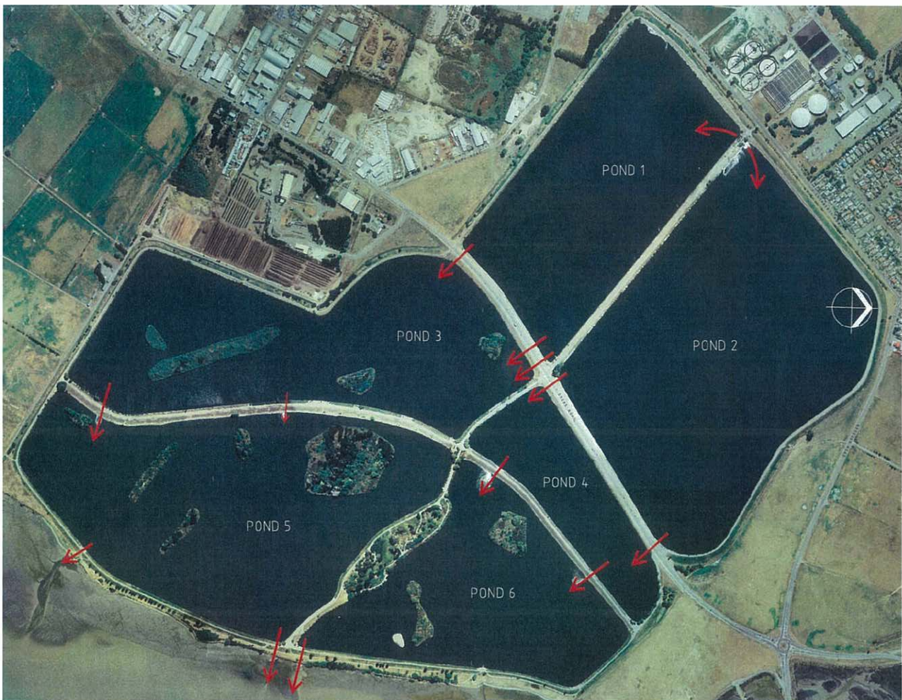
Figure 1: Pond Layout and Flow Paths Before Upgrade
