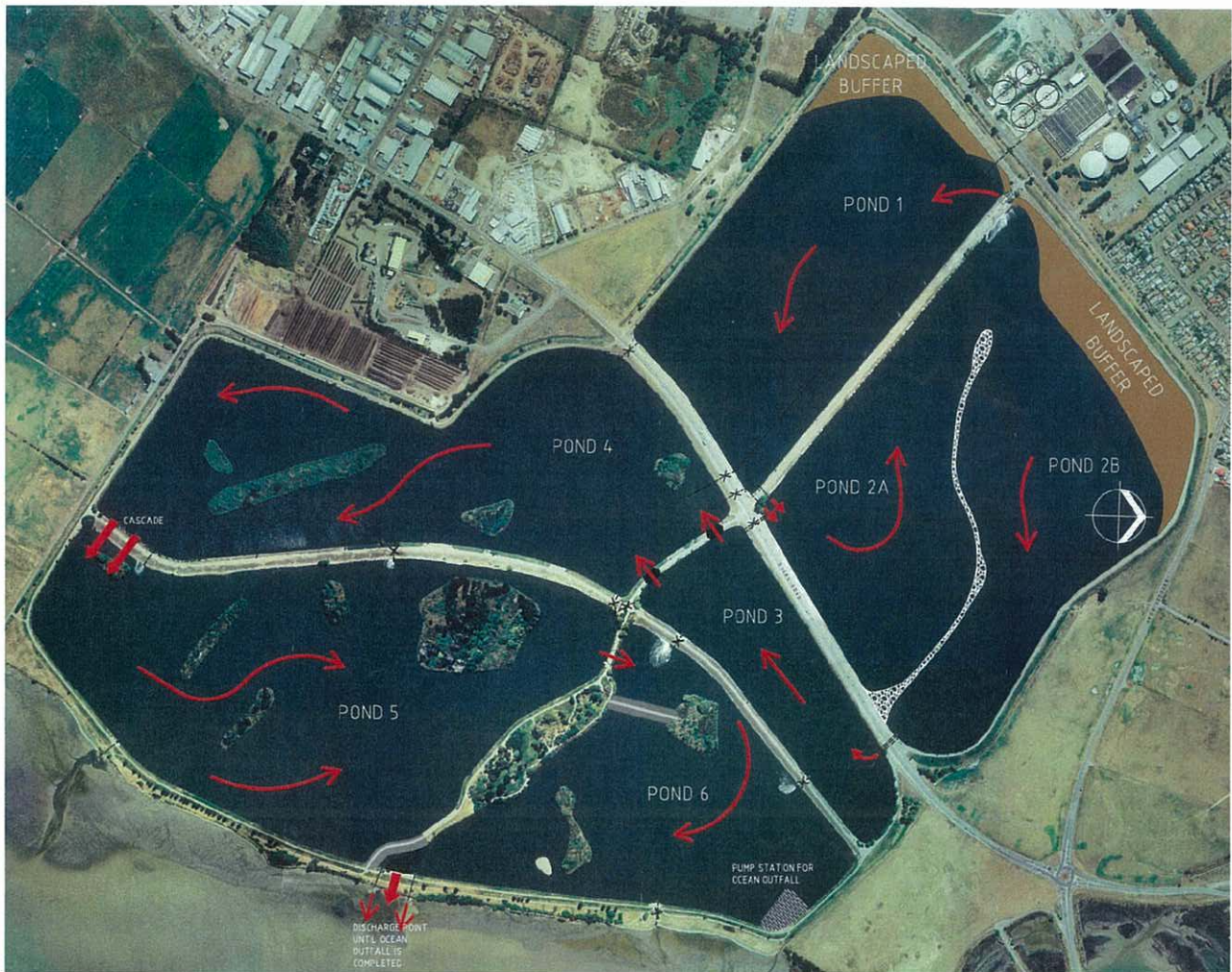
Figure 2: Pond Layout and Flow Paths After Upgrade
