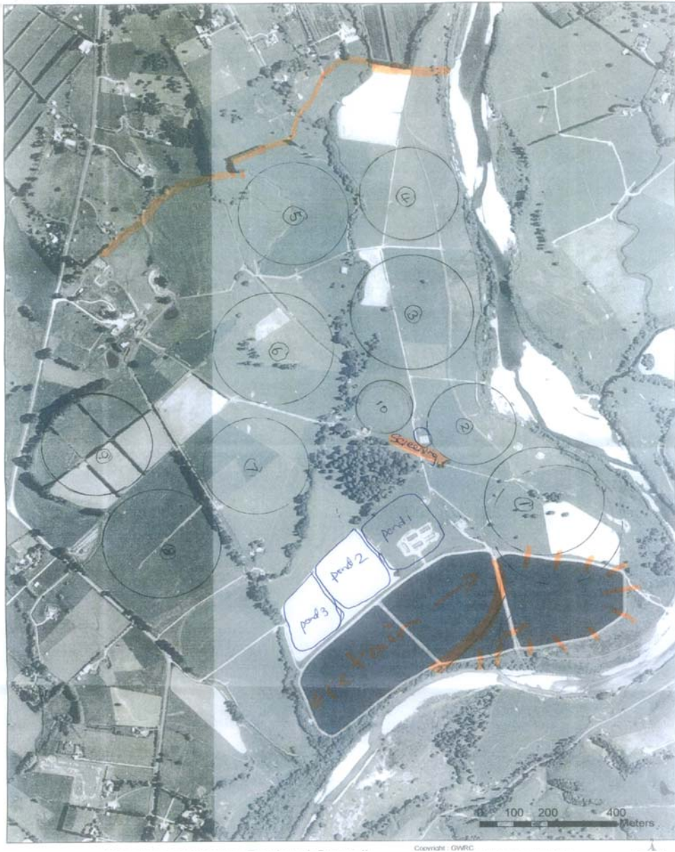
Figure 1 – Forbes Proposal for Ten Centre Pivots Covering 84ha (as supplied by S Forbes)
